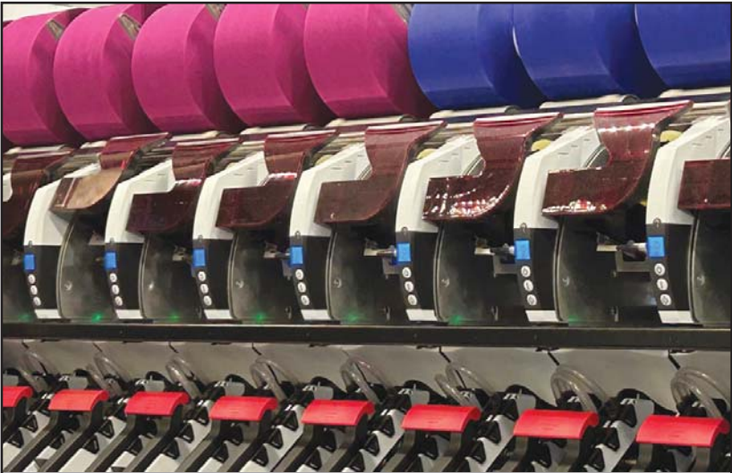
Autoairo air-jet spinning machine from Saurer, for spinning perfect terry towel yarns.
