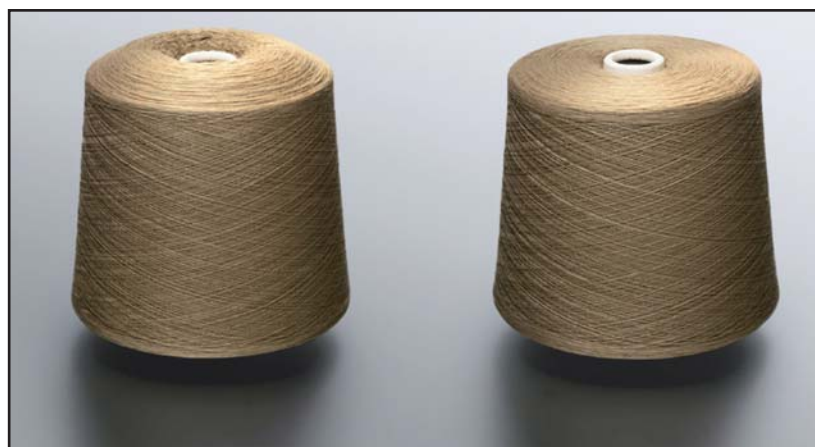
Fig. 3: Superb package with straight flanks (right) thanks to Variopack FX
