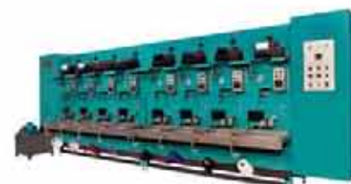
Single End Sizing RI M 8001 (1-4-8 Spindles / Speed 250 MPM)
