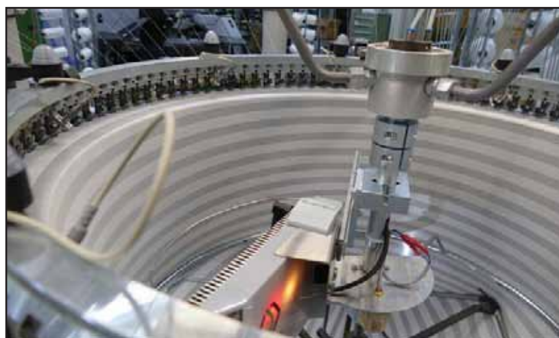
knithawk is a tool for optical defect detection. He sits directly at the knitting point.
