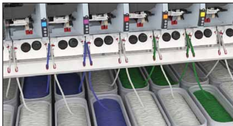
Autocoro 11 rotor spinning station will show the new concept for Duo Sliver Feeding.
