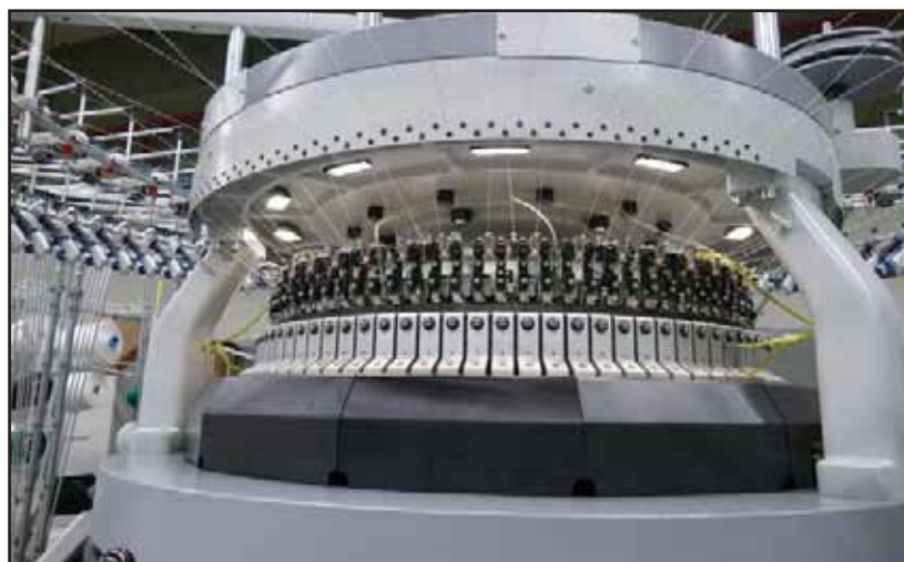
The OVJA 2.4 EC II is equipped with a new system for electronic single needle selection; one of the advantages is a significantly lower knitting head.
