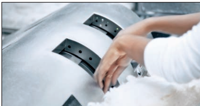
Measuring fiber quality parameters with Uster HVI
